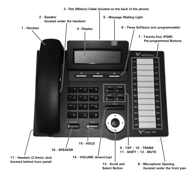
**Note:** The Edge 700 - 24 module phone can have full duplexing capability when the appropriate duplexing module is connected (see item 3 above and on next page)
